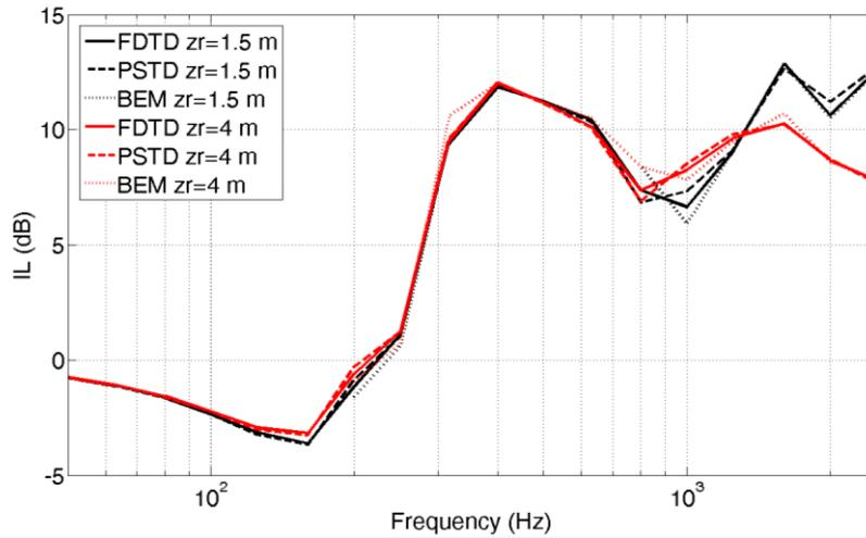
Figure 2 – Parallel wall insertion loss in absence of wind, calculated with FDTD, PSTD and BEM, at the low and high receiver position.
